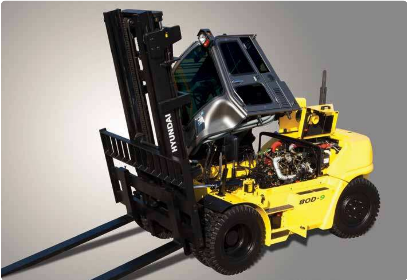
Tilting Cabin & Large Engine Hood Highly accessible engine compartment assures fast and efficient maintenance.
